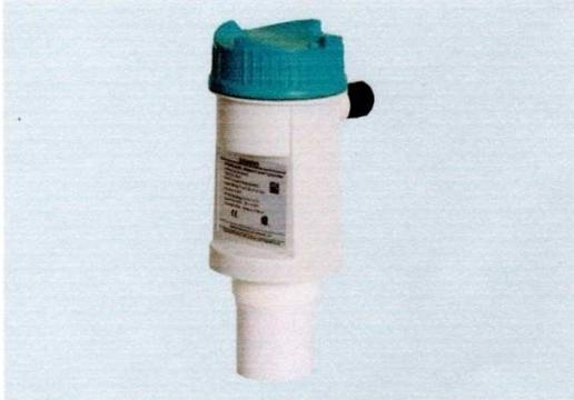
SITRANS LU150 is a short-range integrated ultrasonic level transmitter. This general purpose, 2-wire, 4 to 20 mA loop powered transmitter is ideal for liquids, slurries, and bulk materials in open or closed vessels to 5 m (16.4 ft).
